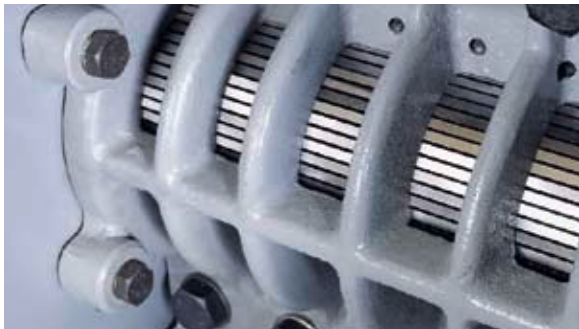
Strainer cage of an oil press with extremely wear-resistant replacement parts.
